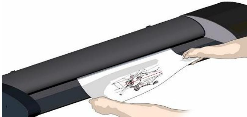
Load the paper, face up. Hold with both hands and align the document's center with the scanner center marking.
