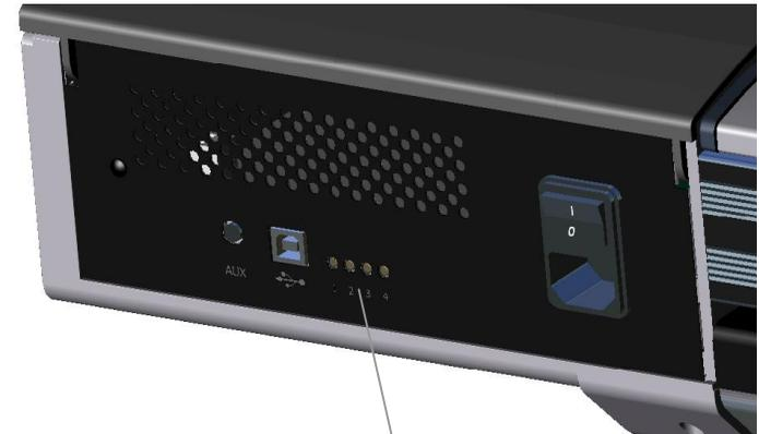
*4 diagnostic LEDs at the scanner back*
