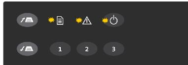
All LEDs are on during self-test
