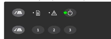
Scanner in **Wake** mode – Power LED is green
