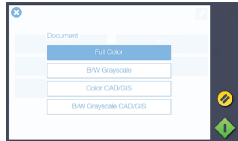
Full Color (selected), B/W Grayscale, Color CAD/GIS and B/W Grayscale CAD/GIS options for scanning a Document to file.
