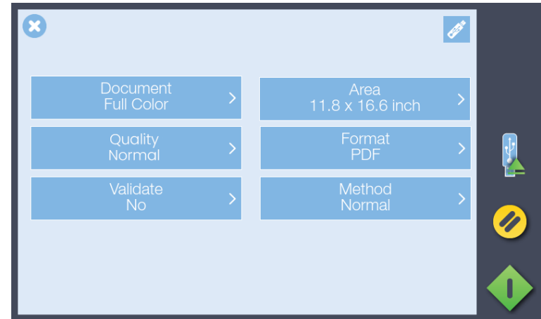
MENU to change: Document Color, Scan Area, Scan Quality, File Format and Validate SCAN options.
