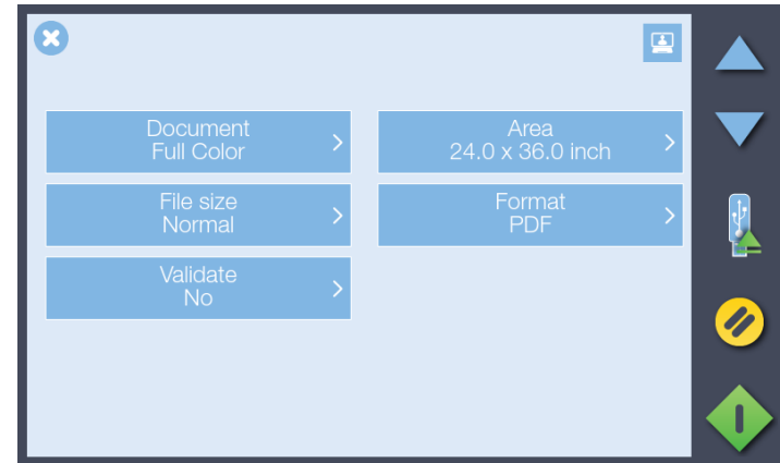
(Above) Menu to change Document Color, Scan Area, Scan Quality, File Format and Validate (annotate) scan.
