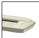
Lift the scanning area lid to access the smart card
